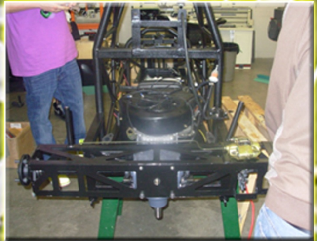
View of the rear end with gear box and engine mounted in.
