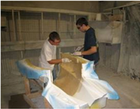
Matt laying up fiber glass into the pre-made mold.
